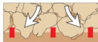
Fig. 1 Interlocking effect of the geogrid with soil
